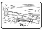
4: Undo clip at both ends of housing. (See 6:)
